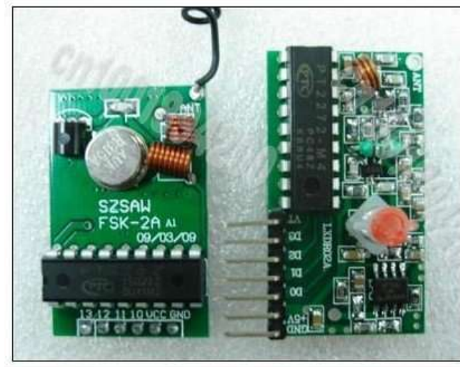
Figure 3 RF Transmitter and Receiver modules
